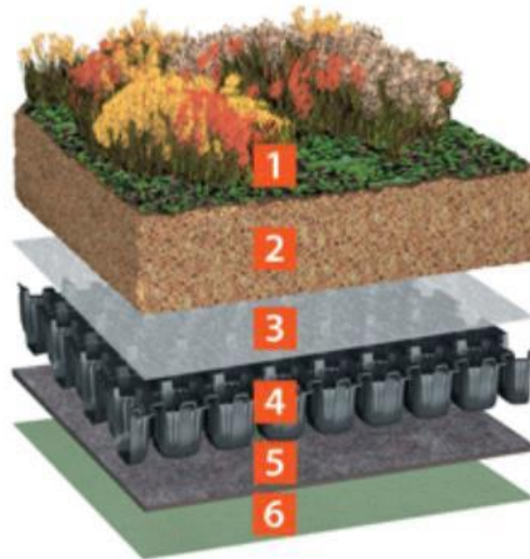
Figure 2 –Typical Extensive Green Roof
